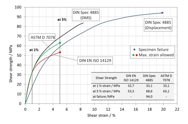
Experimental average in-plane shear stress-strain curves concerning different test methods.
