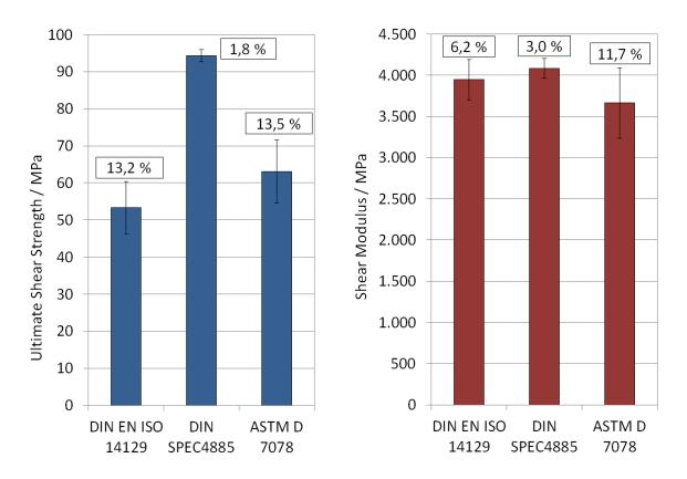
Comparison of shear strength and shear stiffness obtained through different test methods.
