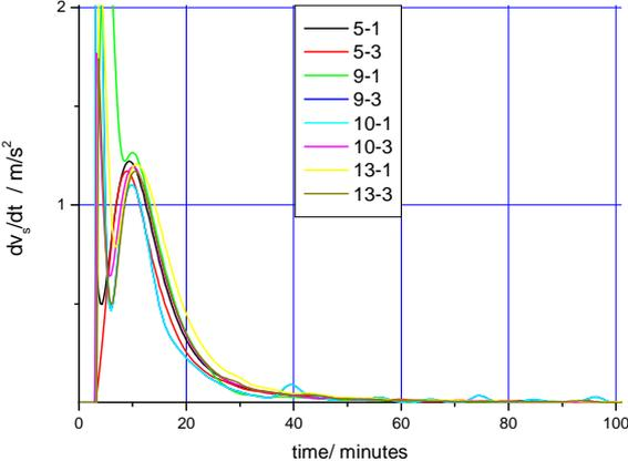
Fig. 6: First deviation of the velocity ( $dv_s/dt$ ) as a function of time. Often it is called “reaction rate”.
