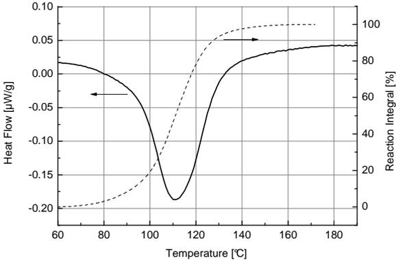
Fig. 7: Heat flow vs. temperature for a T-ramp (1 K/min). From this heat flow the reaction integral is determined.
