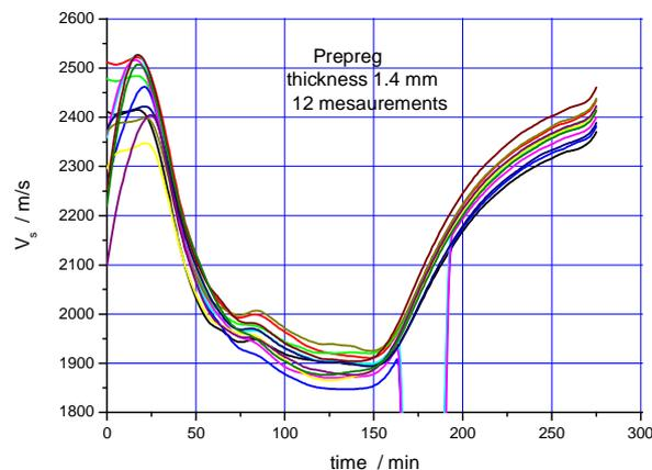
Fig. 3a: Velocity of sound versus time (temperature as function of time in Fig. 3b) for epoxy resin prepreg: 12 separate measurements at the same material showing differences in the absolute value ( $\pm 50$  m/s), but the same characteristic behaviour.
