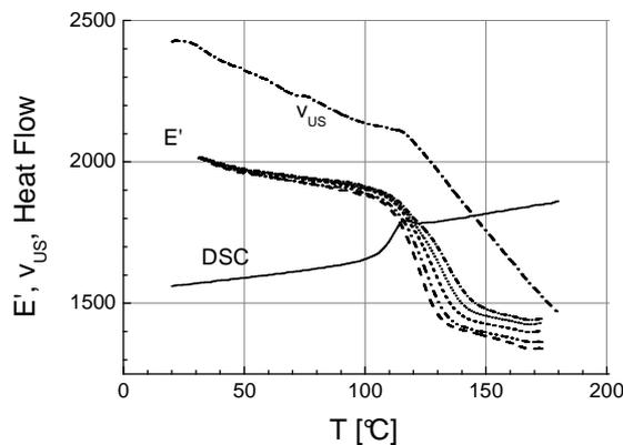
Fig. 10: Signals of three diagnostics vs. time for a T-ramp (1 K/min).  $T_g$  is indicated by all methods.
