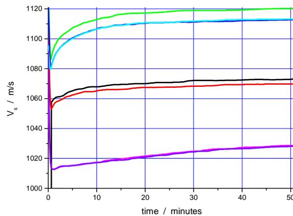
Fig. 5: Isothermal vulcanisation for 3 different rubber samples.
