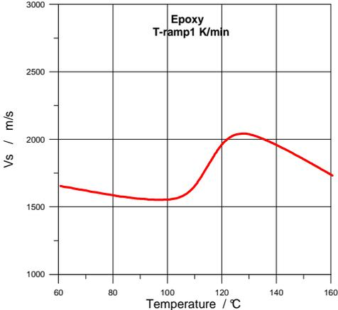
Fig. 8: Ultrasonic speed vs. temperature for the same epoxy resin as in Fig.7
