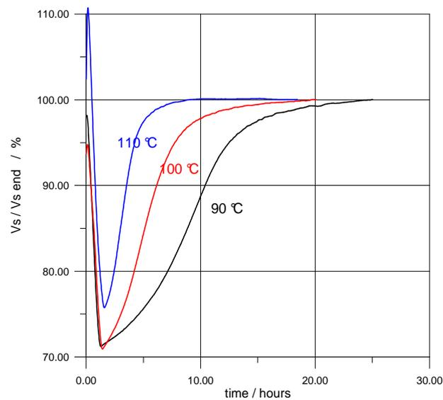
Fig 2: Isotherm curing process of epoxy resin for three different temperatures.
