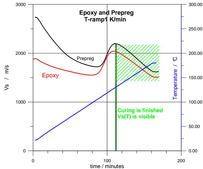
Fig. 4: Velocity vs. time for a T-ramp of 1 K/min. The pure epoxy and a prepreg made with the same epoxy show the same behaviour. Cross linking begins at about 100 °C and is finished at 130 °C.
