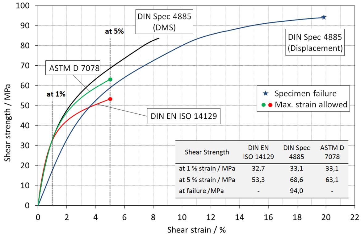
*Experimental average in-plane shear stress-strain curves concerning different test methods.*
