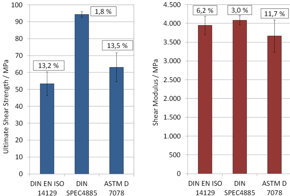
*Comparison of shear strength and shear stiffness obtained through different test methods.*
