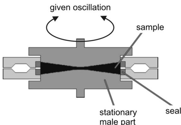
Fig. 1. Functional diagram of the die of a curemeter.
