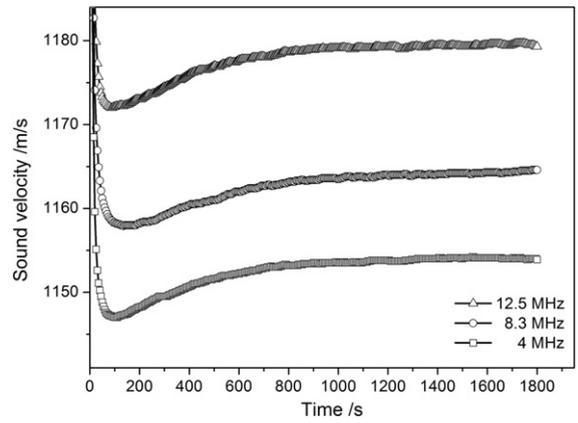
Fig. 6. Sound velocity over time at the crosslinking process, using the parameter ultrasonic frequency, mould temperature 140 °C.
