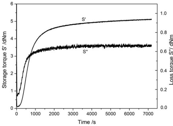
Fig. 4. Storage ( $S'$ ) and loss torque ( $S''$ ) over time, mould temperature 140 °C.
