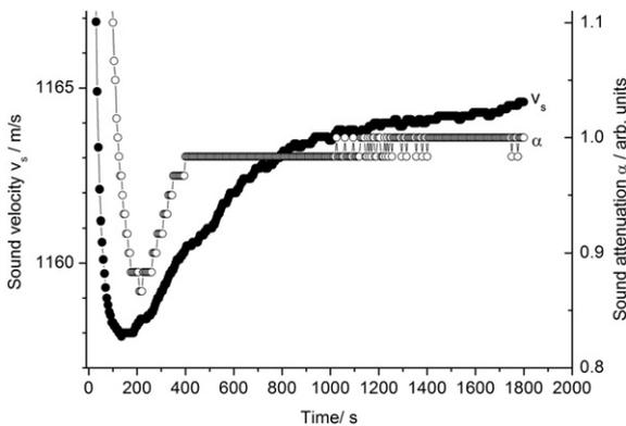
Fig. 5. Sound velocity and attenuation over time at the crosslinking process, mould temperature 140 °C.
