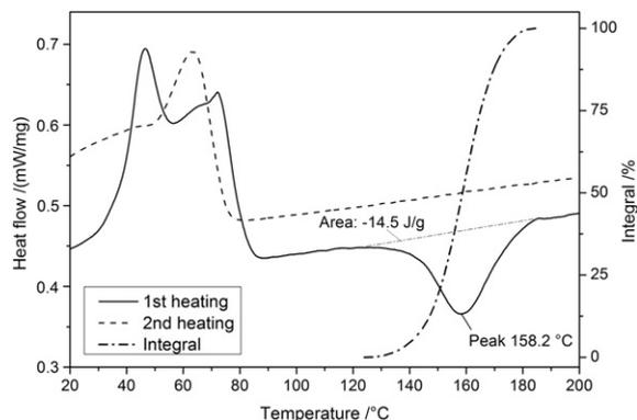
**Fig. 3.** DSC results for 1st and 2nd heating run, reaction integral for exothermic peak in 1st run is included, heating rate 10 K/min.
