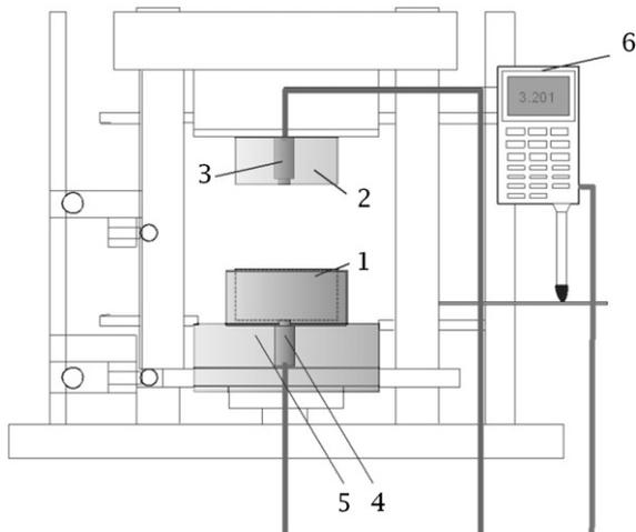
**Fig. 2.** Schematic view of the ultrasonic measuring unit incorporated into a moulding press: 1. and 2. Compression mould, with 3. and 4. incorporated ultrasonic sensors through transmission arrangement, 5. movable rack, 6. thickness dial gauge.
