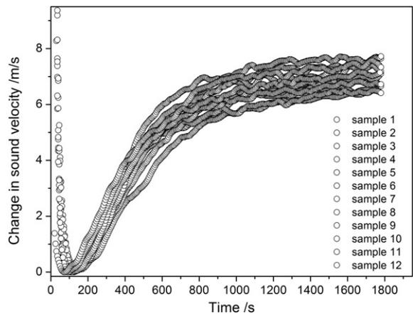
Fig. 7. Change in sound velocity over time at the crosslinking process – test of reproducibility, mould temperature 140 °C.
