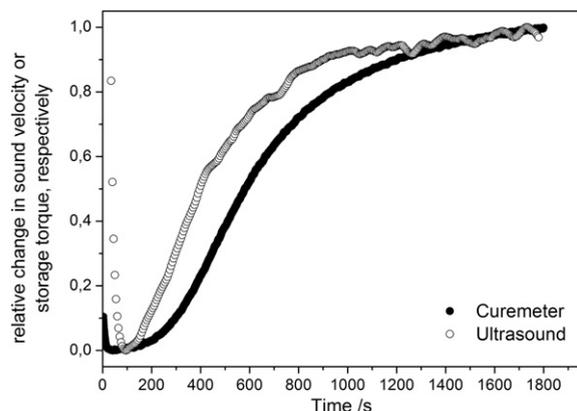
**Fig. 8.** Comparison of change in sound velocity and curemeter storage torque  $S'$  over time at the crosslinking process, mould temperature 140 °C.
