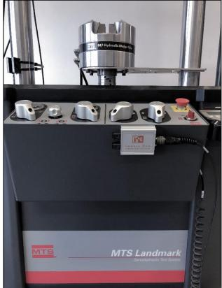
The cable to the measuring amplifier is connected to the strain gauge connection box via an Amphenol socket (push & turn). For the Wheatstone bridge, high-quality and selected supplementary resistors are used. The strain gauge connection box is attached to the frame of the universal testing machine via magnetic feet.
